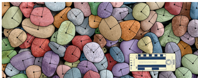
Example of an output from segmenteverygrain https://github.com/zsylvester/segmenteverygrain
