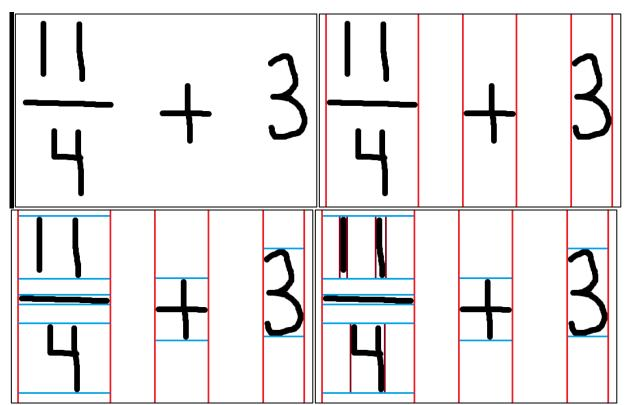
The result is an ordered set of atomic symbols. Though the user is still restricted due to the bounding box effect, we have opened the segmentation up to extension. Since the bitmap is static, the user is not bound by time and may freely go back and edit the equation. Additionally, the vertical scan gave us additional knowledge about the symbols being written.
