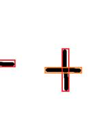
If they cross, we combine the strokes into a single stroke array and find its new bounding box. If the character is not a multi-stoke symbol, we check to see if a fraction is formed. We determined that there is a simple fraction if the centroids of two or more strokes create a best-fit line with an absolute angle greater than 6°. Once a fraction is determined, the strokes comprising it are joined into a single stroke. All remaining strokes are considered atomic and sent to the OCR.
