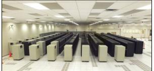
The above machine occupies about 1/3 acre and has 8000 processors, and 400 Terabytes if storage. Interconnect networks for existing machines consist of thousands of cables and many thousand parts.
